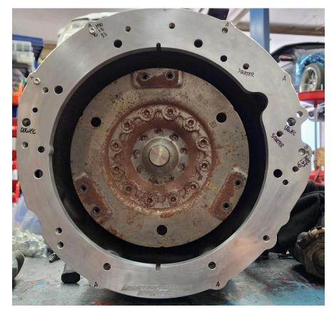
7) Bolting the flywheel to the torque converter
