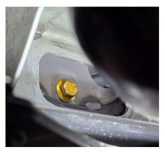
Once the transmission installed, you will now have to bolt up the OEM flex plate to our torque adapter. Using the access hole underneath the engine, insert the 6 supplied M10x1.50x20 bolts in every other hole. Torque to 25 ft. lbs., using red thread locker.
