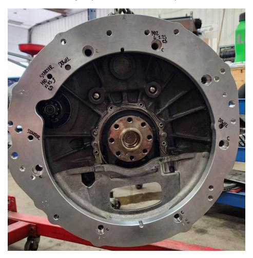
You can now bolt on the adapter kit using the supplied M12 Allen bolts in the countersunk holes (marked "C" on the picture above). The two slightly shorter bolts (25 mm instead of 30 mm), are meant to be threaded in the two top boltholes. Torque to 55 ft. lbs.
